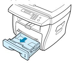
Push down on the pressure plate until it locks into place.
