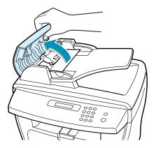
Rotate the bushing on one end of the ADF roller toward the ADF ((a)) and remove the roller from the slot((b)). Pull the document gently to the right and out of the ADF.
