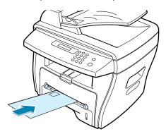
Adjust the paper guide to the width of the print material.
