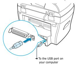
If you want to use a parallel printer cable, only use a IEEE 1284 compliant cable and connect it to the parallel connector on your machine.
