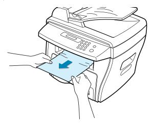
If there is any resistance and the paper does not move when you pull or if you cannot see the paper in the front output tray, open the rear cover.
