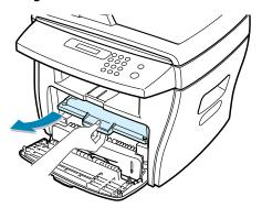
With a dry and lint-free cloth, wipe away any dust and spilled toner from the toner cartridge area and the toner cartridge cavity.
