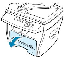
2 Remove the starter toner cartridge from its bag. Gently roll the cartridge to distribute the toner.
