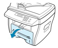
2 Pull the toner cartridge out and gently roll the cartridge to distribute the toner evenly inside the cartridge.
