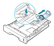
2 After inserting paper into the tray, slide in the guide until it lightly touches the end of the paper stack.
